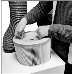
Figure 9: The cartridge may now be removed by holding the lugs and lifting from the extractor.
